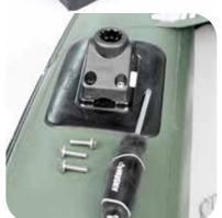
Attach deck mounts with 7/8" screws provided to the pad mounts at the bow & near the transom. Screws are located in Orange Repair Kit.
